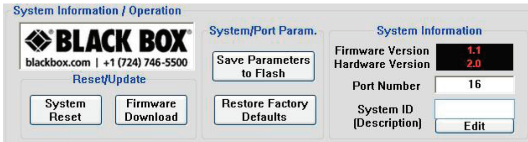
Figure 5-3. System setup, control, information, and port commands.
